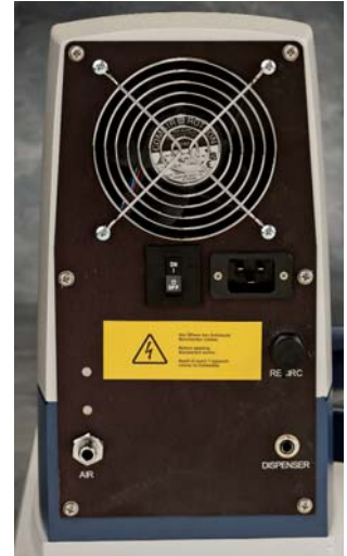
Back control panel contains power button, air inlet, recirc and PriMet® connectors.
