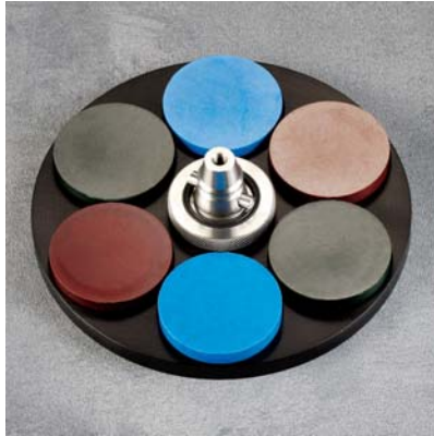
Single force specimen holder and drive adapter.
