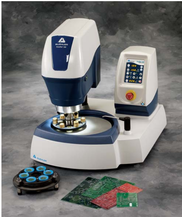
PC Met® Precision Printed Wiring Board Accessory connected to AutoMet® 300 Power Head with central force drive adapter (sold separately).
