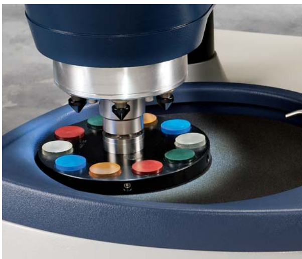
Central force application for superior flatness.
