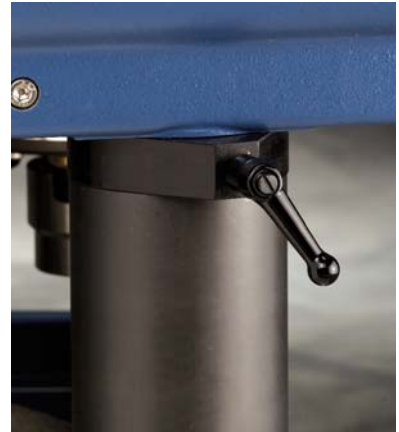
Head position locator stop handle allows specimens to be located at the same position over the platen every time.
