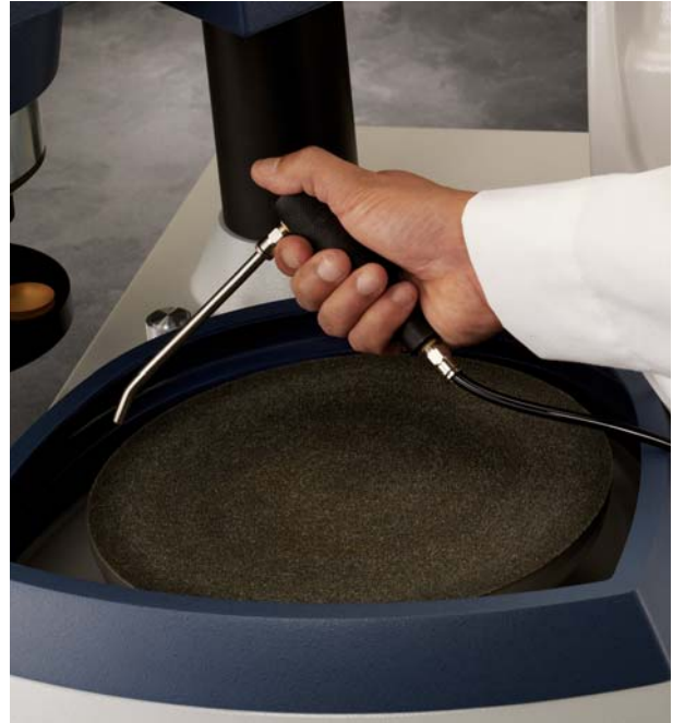
Retractable water hose reaches over entire bowl for ease of cleaning.
