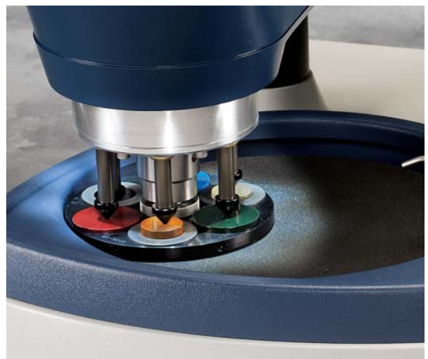
Single force application for preparation flexibility.
